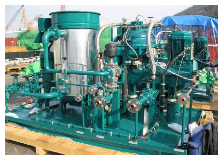
GEA Westfalia – Fuel Oil Separator
